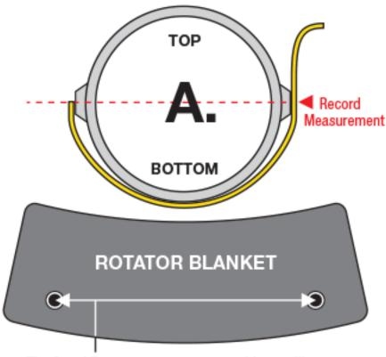
The A and B measurements you provide us will determine the accurate postioning of the gromments on your blanket.
